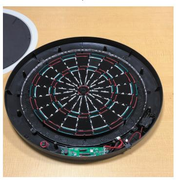
3:Remove the LED connector from the PC board
