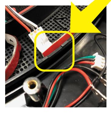
The starting point is recessed one step. Align the tip of the LED strip with the recess.
