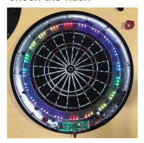
8:Attach rubber mat, sensor sheet, protective mat and back cover.
