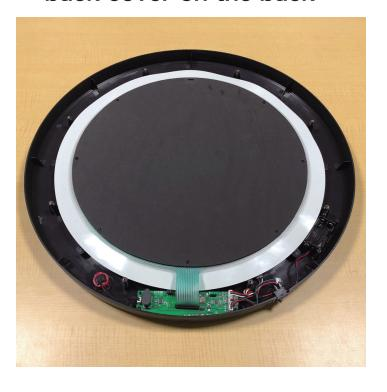
2:Remove the protective mat, sensor sheet, and rubber mat
