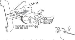
When attaching the holder to the Pole Stand, hold and push the holder to the Pole Stand firmly to avoid a fall and knob it tightly.
